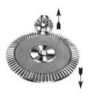
For Spiral Bevel and Miter Gears, the direction of axial thrust loads developed by the driven gears will depend upon the hand and direction of rotation. Stock Spiral Bevel pinions cut Left Hand only, Gears Right Hand only.
