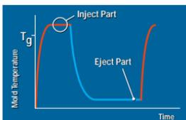
Dynamic thermal cycling — combines structural mass reduction with selective heating and cooling of the mold to improve finished part quality and enable more complex designs
